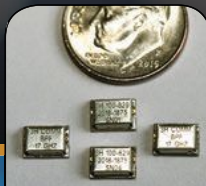
Pico, SMT Filters, available from 5.0 GHz to 27 GHz
